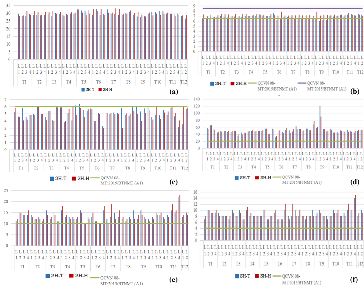
Figure 2. Water quality parameters: (a) Temperature; (b) Values of pH; (c) Concentrations of DO (mg/l); (d) Concentrations of TSS (mg/l); (e) Concentrations of COD (mg/l); (f) Concentrations of BOD 5 (mg/l).
